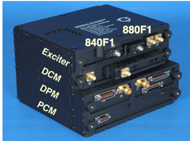
Fig. 2 The Juno Small Deep Space Transponder showing the four modules
