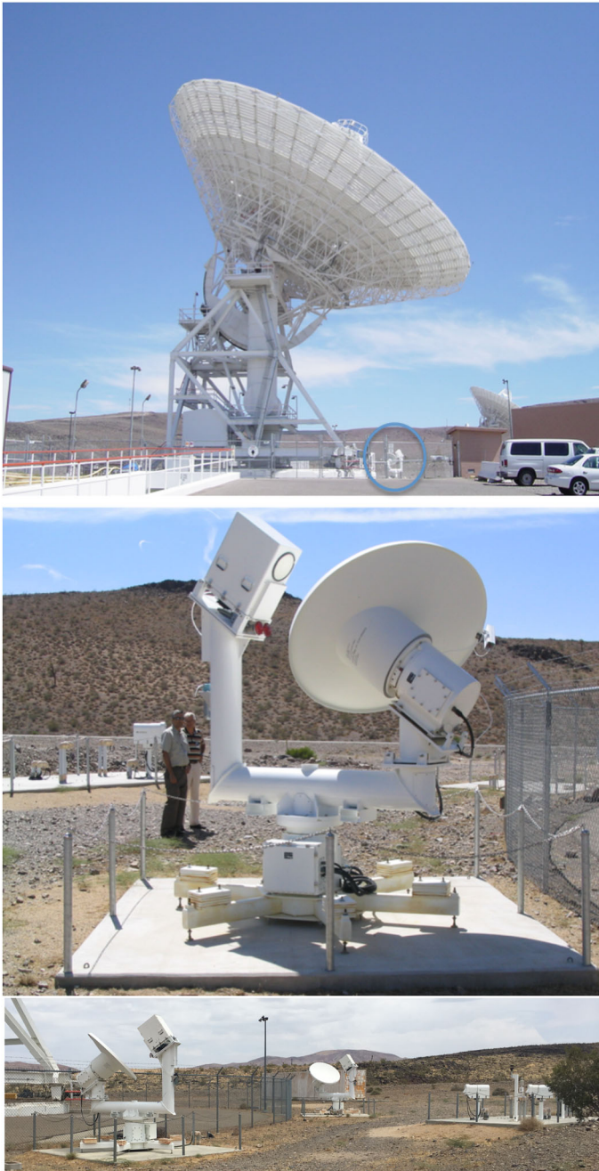
Fig. 6 Upper panel is DSS-25, a 34-m diameter station at NASA's Deep Space Network, Goldstone, California, capable of Ka-band uplink and downlink. In the drawn blue circle is the Advanced Water Vapor Radiometer (AWVR) showing relative location and size to the DSN station. The middle panel shows a close-up of the AWVR showing relative size to personnel. The lowest panel shows the two AWVRs and their Microwave Temperature Profilers (MTP); mounted on the right concrete pad are the surface meteorology packages and wind sensors
