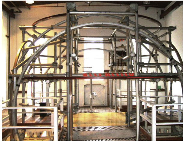
Fig. 25 The 22-foot Braunbeck coil system at the Mario H. Acuña Magnetic Test facility at NASA's Goddard Space Flight Center
