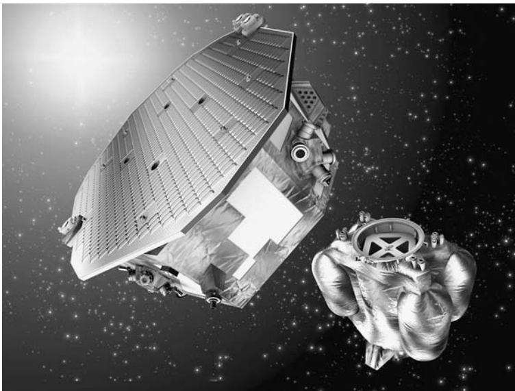
Fig. 7 Artist impression of the LISA Pathfinder after separation of the science module from the propulsion module, before reaching the operational orbit around L1
