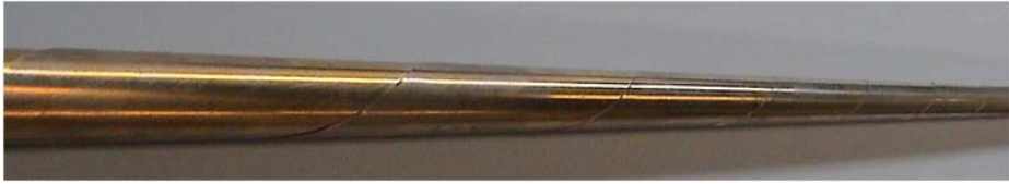
Fig. 6 Beryllium copper stacer antenna element. The aspect ratio is exaggerated here for display purposes
