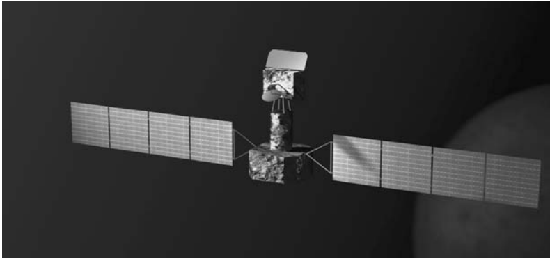
Fig. 13 The configuration of the Colombo (as it was then called) composite on its way to Mercury, comprising the planetary and magnetospheric orbiters, together with the large solar panels of the SEP subsystem. This concept was the outcome of the second industrial study in 1999
