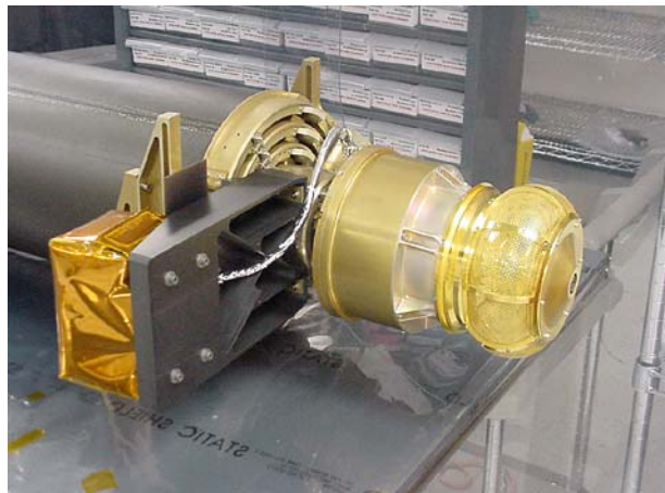
Fig. 4 The solar wind electron analyzer at the end of the stowed IMPACT boom and the magnetometer on its shelf. After boom deployment the two instruments are separated by ~1 m
