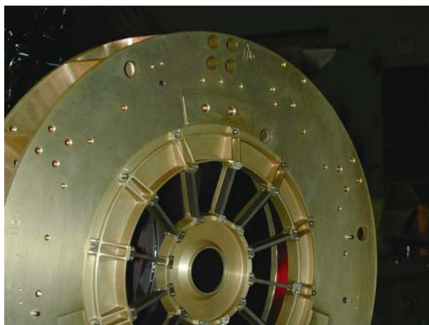
Figure 10. The XRT electron deflector, mounted on the rear face of the OBIF. The electron deflector consists of 12 rare earth bar magnets mounted on radial spokes aligned with the mirror spiders. These provide a high azimuthal magnetic field across the optical path with very low dipole moment.
