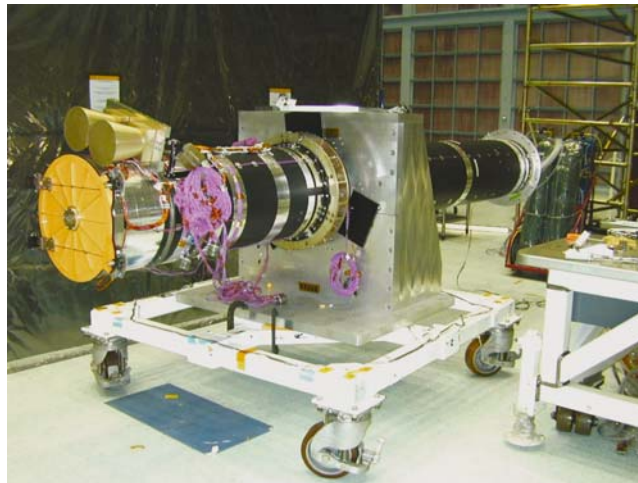
Figure 4. XRT installed in test cart before thermal vacuum tests in July 2002, with star tracker simulators installed. The telescope door is at the left end. The silver bands around the tube are aluminum tape over the operational and survival heaters.
