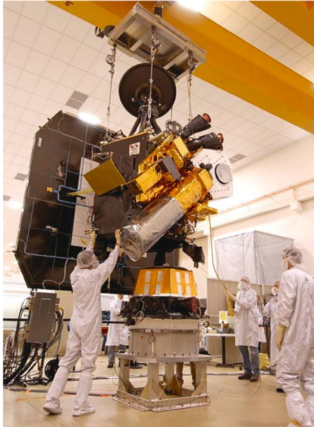
Figure 2. The flyby spacecraft being lowered onto the impactor spacecraft in the clean room at Ball Aerospace and Technologies Corp. prior to system environmental tests. When the spacecraft are joined, the pentagonal gold-colored panels of the impactor are recessed entirely inside the flyby spacecraft. The white ring at the bottom of the impactor, here bolted to the top of a test stand, is the fixture that will join the impactor to the launch vehicle. Photo courtesy of Ball Aerospace and Technology Corporation.
