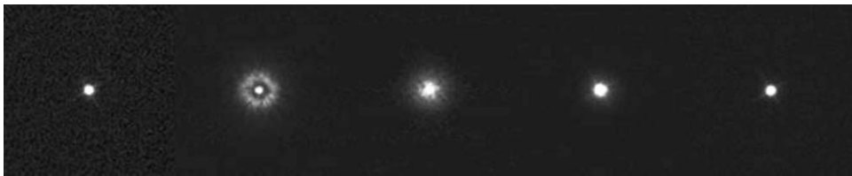
Figure 33. The figure above show stellar images taken before the anomaly, one image taken after the anomaly surfaced, and three taken after the decontamination sequences, all in the same BL1/CL2 filters and adjusted for total stellar brightness. The images are all contrast enhanced in the same manner to show the faint extended light. All images were taken at a CCD temperature of -90^\circ C. Calculations indicate that for this filter combination, approximately 68% of the light fell outside a radius of five pixels when the anomaly was at its maximum. After the first sequence (third image above), that fraction was reduced to 44%; after the second (fourth image above), 18%. It is now 5% (fifth image above). . . back to pre-anomaly values.
