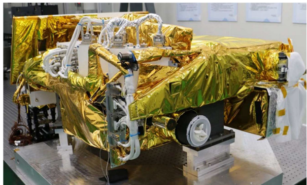
Figure 5 The flight model of LST (dimensions: 1380 mm \times 818 mm \times 474 mm).
