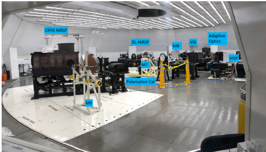
Figure 10 Coudé rotator with instrument beam distribution optics and instruments. The picture was taken during the instrument integration process. The VTF will be added in early 2021. The diameter of the rotator is 16.5 m.
