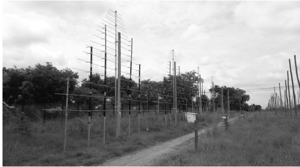
Figure 4 Image of a single group. The antennas are nearly 6 m tall and 5 m wide. The smaller antennas on the far side are a part of the GRIP array.
