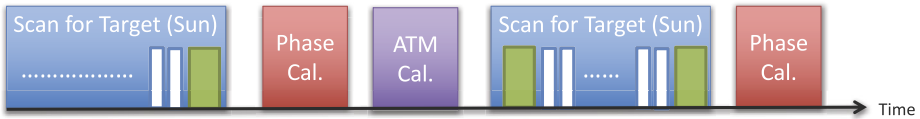
Figure 4 A cartoon of the observing sequences around a scan of a target. A box indicates the period of a scan. A scan is constructed from multiple subscans as shown in the “Scan for Target”. Except for the scan for target, subscans are omitted in the figure. A red box indicates a scan for the phase calibrator; a blue box is the scan for the scientific target, and a purple box indicates a scan for atmospheric calibration near the target. White narrow boxes indicate subscans of observing the target, and green boxes indicate subscans of observing sky near the Sun with the attenuating levels for observing the Sun.
