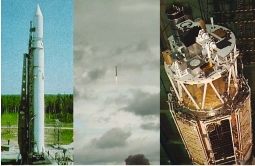
Figure 1. Left: The Cyclone SL-14 rocket on the launch pad at the Plesetsk Cosmodrome, northern Russia, on the morning of the launch, 31 July 2001. Centre: The cyclone rocket shortly after launch. Right: The instrument payload of CORONAS-F: the spacecraft is \sim 1.5 m in diameter and weighs \sim 2.5 tonnes. See Figure 3 for location of the RESIK instrument.
