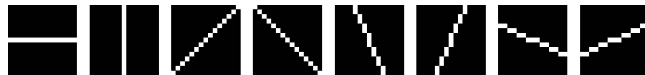
Figure 2. The eight directional 15 \times 15 pixels linear structuring elements used by the advanced morphological filter to remove spurious pixels from the filaments mask. White pixels have value 1 and back are zeroes.
