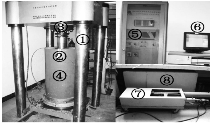
Fig. 1. Test equipment: 1) loading frame, 2) displacement sensor, 3) load sensor, 4) triaxial chamber, 5) main operating system, 6) data acquisition system, 7) confining pressure loading device, 8) normal force loading device.
