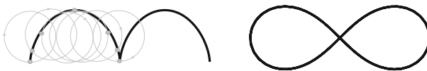
Fig. 3 Two important curves connected to the development of mathematics, the Cycloid (left) and the Lemniscate of Bernoulli (right). The Cycloid is the curve traced by a point on a rolling circle
