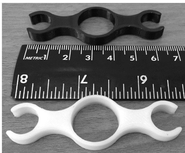
Fig. 2. POM- and graphitized CNT/POM-based cable clamps fabricated using a 3D printer.
