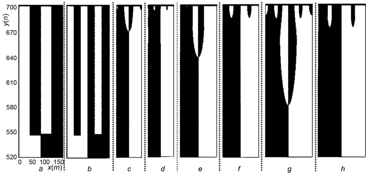
Fig. 3. Initial configurations of wrinkles \{1 \rightarrow 2\} (a) and \{1 \rightarrow 3\} (b) in the nanoribbons and configurations formed as a result of relaxation for the calculated areas of various sizes: c, d - L = 126.56 \text{ \AA} , e, f - L = 180.8 \text{ \AA} , g, h - L = 235.04 \text{ \AA} . For c, e, g, the transitions \{1 \rightarrow 2\} are formed and for d, f, h, the transitions \{1 \rightarrow 3\} are formed. Black (white) color corresponds to a positive (negative) displacement of atoms from the nanoribbon plane.
