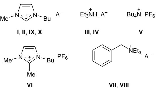
**I, III, A = BF<sub>4</sub>; II, IV, A = PF<sub>6</sub>; VII, IX, A = AlCl<sub>4</sub>;**
