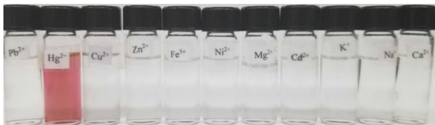
Fig. 2 Colorimetric changes of RD6g (20 \mu\text{M} ) upon the addition of 10 equiv. of various metal ions in \text{CH}_3\text{CN}/\text{H}_2\text{O} (9:1 v/v) at room temperature
