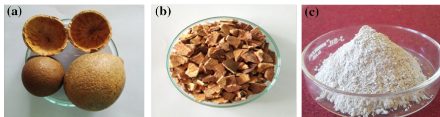
Fig. 2 a Dry bael fruit rinds. b Small pieces of bael. c BFA catalyst
