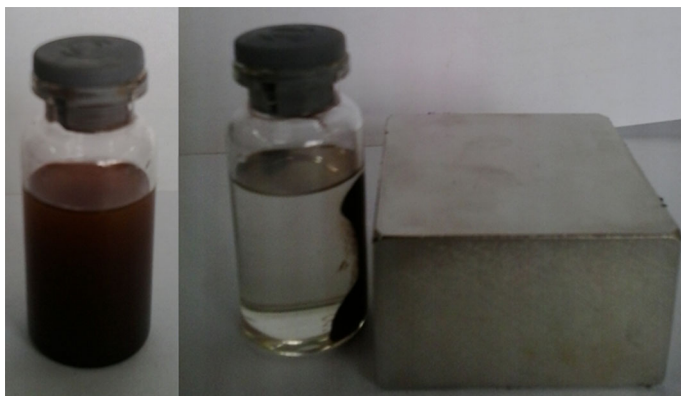
Fig. 8 Image showing SA-PYCA-Fe 3 O 4 nanoparticles can be separated by an applied magnetic field. A reaction mixture in the absence ( right ) or presence of a magnetic field ( left )
