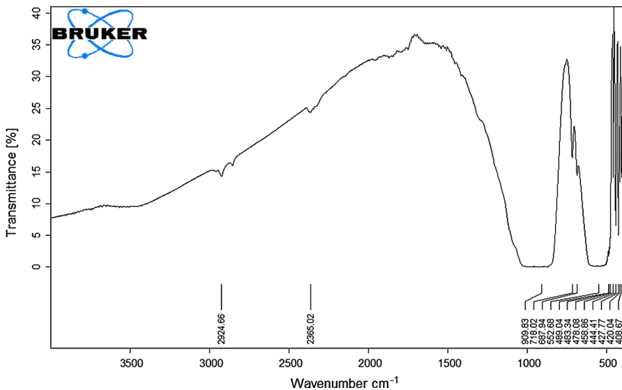
Fig. 3 FTIR spectra of Y_2SiO_5:Ce^{3+}
