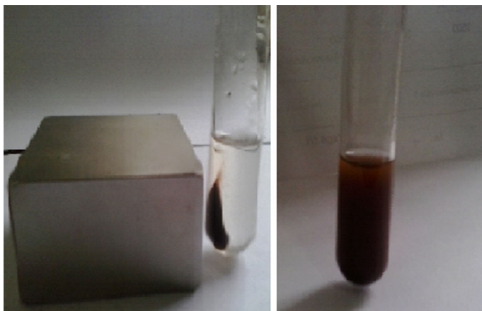
Fig. 7 Image showing that \text{Fe}_3\text{O}_4 -PYCA nanoparticles can be separated by an applied magnetic field. A reaction mixture in the absence ( right ) or presence of a magnetic field ( left )
