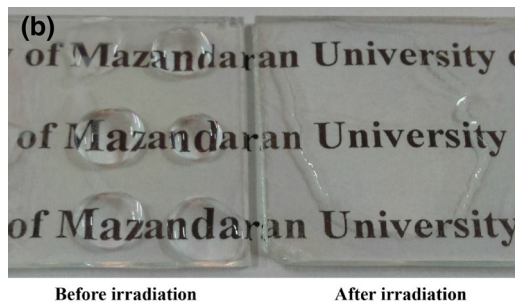
Fig. 7 a Changes in the contact angle of the water droplet under visible light irradiation on TiO 2 NLS with various silver contents and b optical image showing the hydrophilicity behavior of Ag-TiO 2 NLS before and after visible light irradiation
