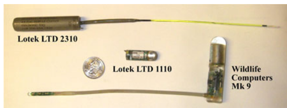
Fig. 1 The three varieties of electronic archival tag implanted into Pacific halibut. All tags recorded temperature and depth; the LTD 2310 and Mk9 also recorded light-levels (irradiance) via a stalk protruding externally through the fish's eyed-side peritoneal wall. An American quarter dollar is added for scale
