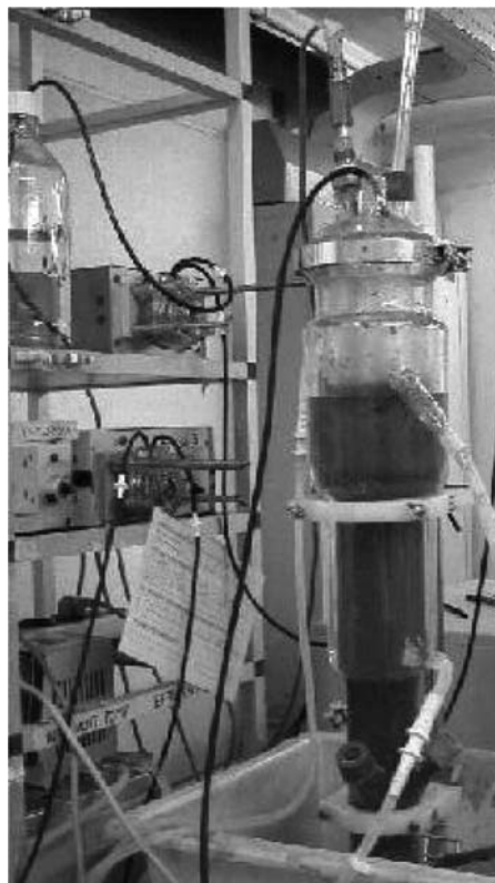
Figure 2. CANON oxygen-limited gas lift reactor in which aerobic ammonium-oxidizing bacteria and anammox bacteria cooperate to remove ammonium directly into dinitrogen gas (Sliemers et al. 2003).
