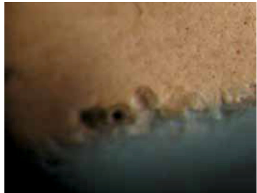
Fig. 3. Corrosion pits on the edges of the specimen with an oxide-ceramic coating. 10×.
