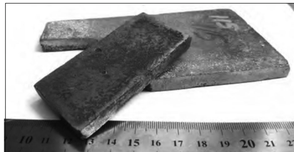
Fig. 1. Plates obtained by free SHS-compression method.
