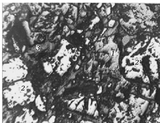
Fig. 3. Refractory working zone microstructure after operation in electric furnace arch: 1) periclase; 2) changed chrome spinelid; 3) secondary spinels; pores are dark. Reflected light. \times 210 .
