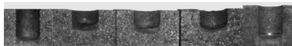
Fig. 5. Chromium-bearing refractory specimens after test in basalt fiber liquid. From left to right: KhKT-10, KhKT-30, KhKT-45, KhKT-60, KhS-MVU.
