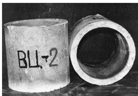
Fig. 5. Fusion-cast ring components prepared from a high-zirconia refractory material.
