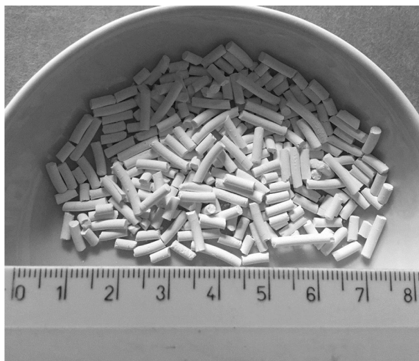
Fig. 2 Hydrotalcite extrudates—a photo with a ruler (cm)
