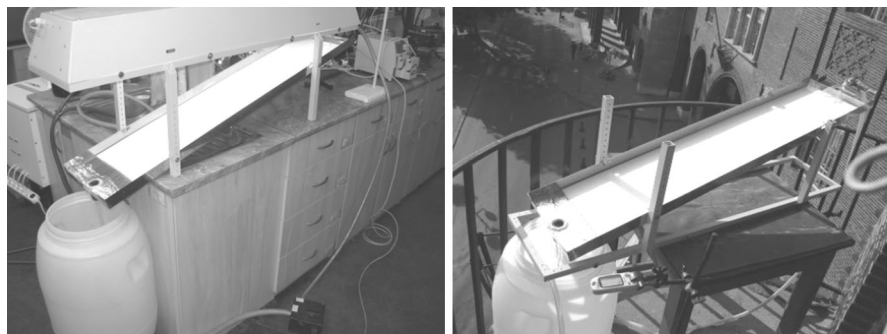
Fig. 9 Photograph of pilot-scale flow reactor with (a) and without (b) artificial irradiation (semiconductor particles were activated by solar radiation)
