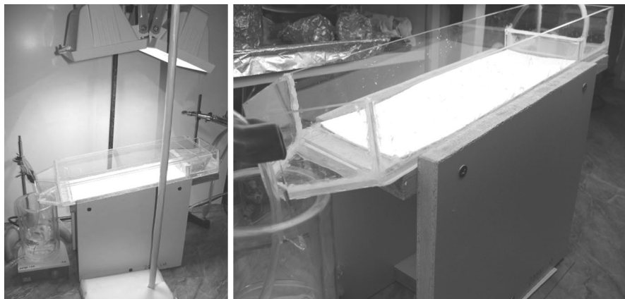
Fig. 1 Photograph of laboratory-scale flow reactor applying immobilized \text{TiO}_2 photocatalyst, equipped with visible light-emitting halogen floodlight reflectors (a) and UV-A fluorescent tubes (b)
