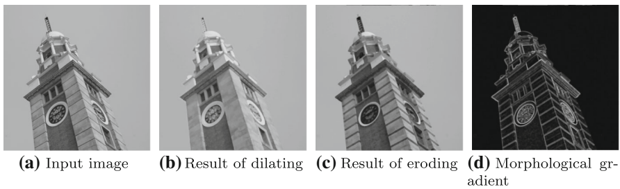
Fig. 28 Example of edge detection
