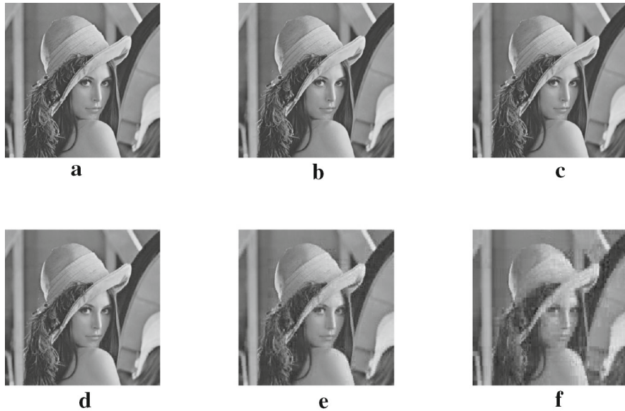
Fig. 8 Original Lena image and recovery images. a The original image of 512 \times 512 . b–f The recovery images by selecting the largest SD coefficients of 2^{16} , 2^{15} , 2^{13} , 2^{11} and 2^9
