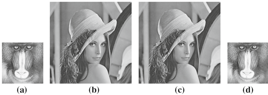
Fig. 12 Example of proposed scheme (carrier image: Lena watermark: mandrill), a watermark, b carrier image, c watermarked image, PSNR = 43.85 d extracted watermark PSNR = Inf
