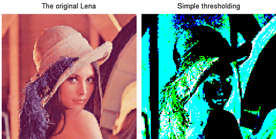
Fig. 15 The experiment 4.a : lena and lena after threshold processing result: pr(1) = 0.4413 , SIM = 0.1174
