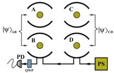
Firstly, an auxiliary photon is sent to interact with the atom confined in the cavity  $D$ , leading the state of the entire atom-photon system to the form
