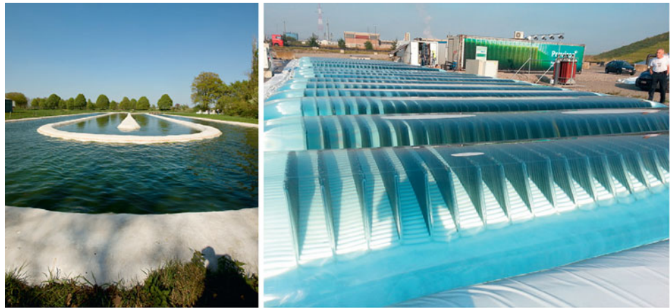
Fig. 2 Pictures of a raceway pond in Ingrepro, The Netherlands ( left image ) and a low-cost photobioreactor in Proviron, Belgium ( right image ). Reprinted with Elsevier permission from Vandamme et al. (2013)
