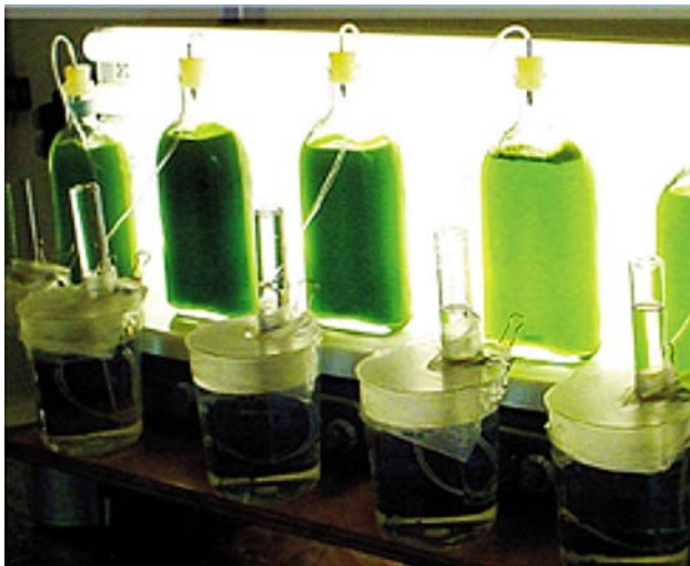
Fig. 5 H 2 -production measurements of S depleted green algae in the laboratory using gas traps. The gases produced by the algae are collected in inverted graduated cylinders via the water displacement method. Samples of the gas can be removed utilizing syringes with long and bended needles. As the cells pass into the H 2 -producing phase, yields of H 2 can be measured directly from the volume of the water displaced in the graduated cylinders
