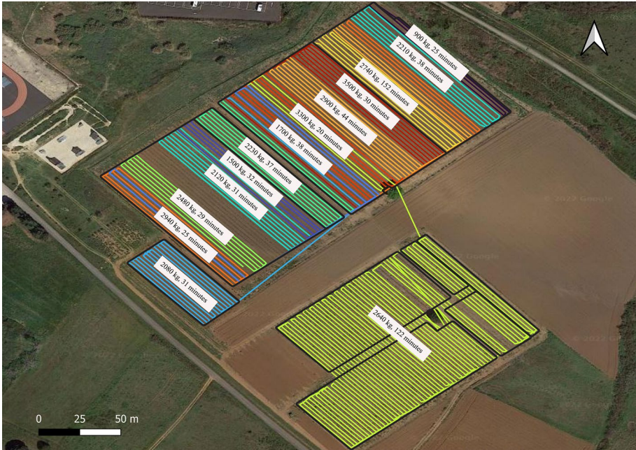
Fig. 2 Example of intra-blocks grape harvester path recorded within some vineyard blocks over the harvesting season. The black lines correspond to block boundaries. Each color corresponds to a harvest sector associated with a WE. Mass of grapes and harvest time duration associated with WE s are displayed on the map
