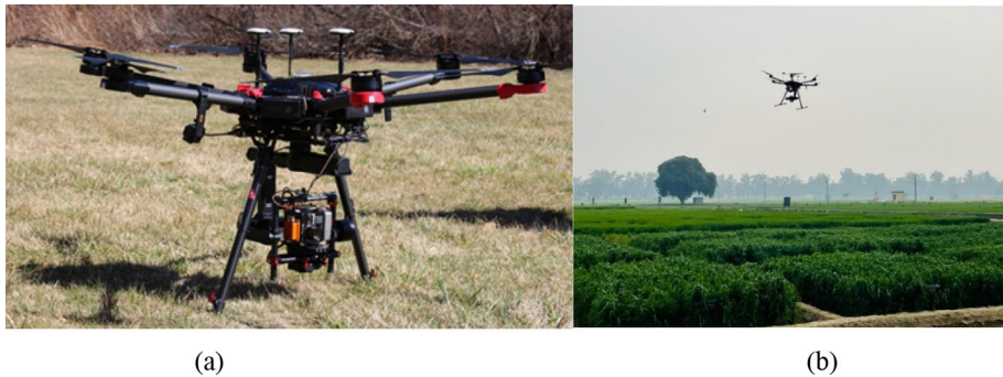
Fig. 2 a Drone with hyperspectral camera facing nadir, b image data acquisition in wheat field
