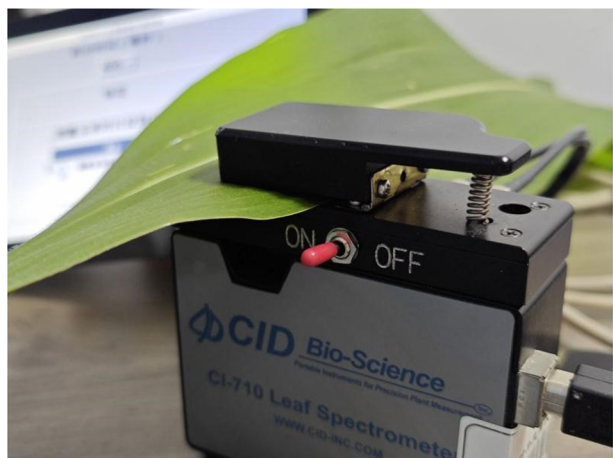
Fig. 1 The portable CI-710 fiber spectrometer to measure the reflectance spectrum of a sugarcane leaf
