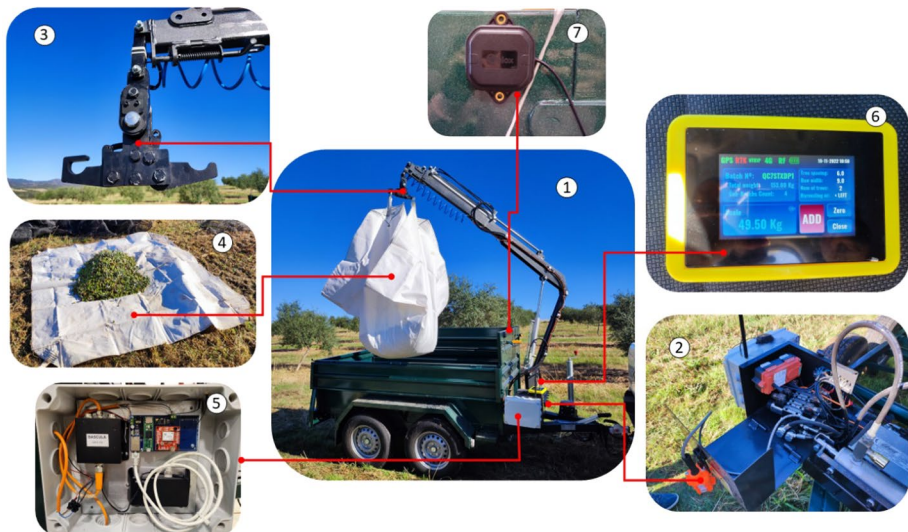
Fig. 1 Components of the yield monitor. 1 Transport trailer, 2 Electronic and hydraulic system for arm control, 3 Implement with loading bolt for weighing fruit, 4 Standard big bag for loading fruit, 5 Electronic system for geo-referencing fruit big bags, weighing and sending data, 6 Wireless electronic system for logistic configuration and visualisation, 7 RTK GNSS antenna
