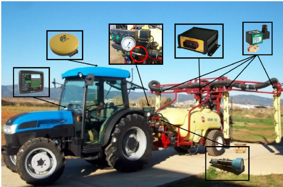
Fig. 2 Variable rate application prototype
