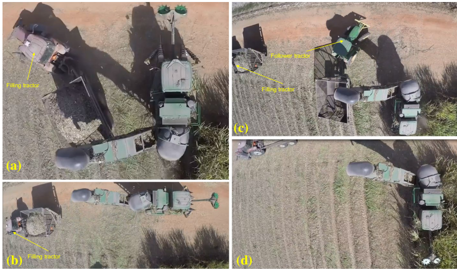
Fig. 4 Tractor and harvester turning procedure: a The tractor is exiting the row and traveling on the headland, b the harvester is completing a 180° turn, where the rotational direction of the toppler blades is reversed and the elevator is rotated to the opposite side of the harvester, c the follower tractor approaches the harvester, d the harvester waits for tractor to enter the row and initiate filling the wagon
