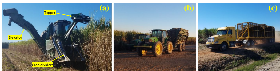
Fig. 2 Harvesting green sugarcane near Edgard, Louisiana. a John Deere 3520 sugarcane harvester, b tractor pulling 10 Mg high dump sugarcane wagon, and c loaded semi-truck en route to the sugar mill (Color figure online)
