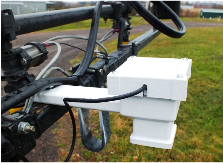
Fig. 3 Custom developed camera enclosure and mounting arm attached to rear sprayer boom for image acquisition
