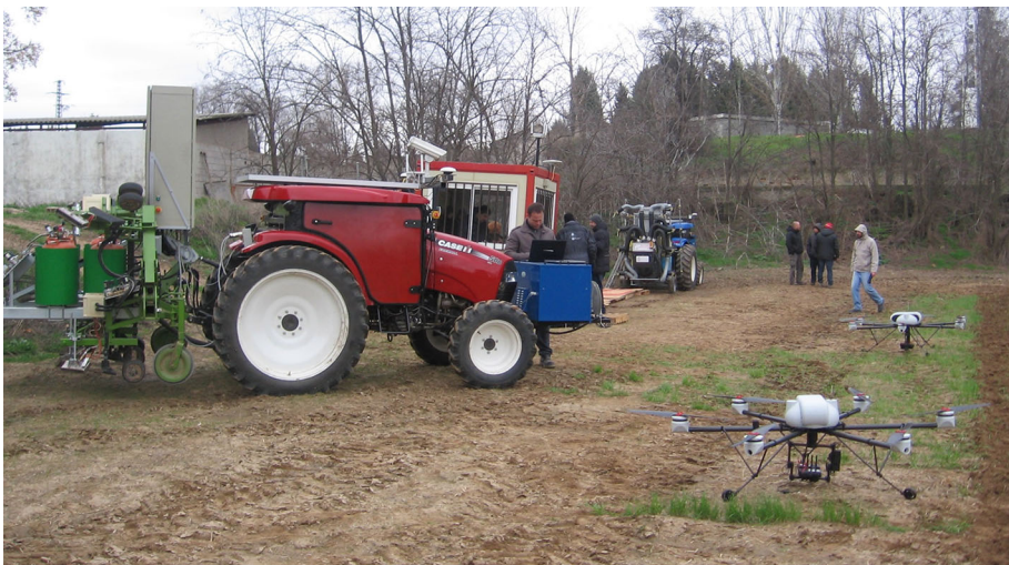
Fig. 1 The RHEA fleet: UGVs and UAVs
